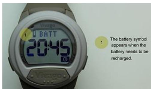
Figure 7. Vivago CARE watch indicates with the battery symbol when the battery is nearly empty
