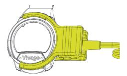
Place the charger on the device as shown on the picture and plug the charger into a power socket.
