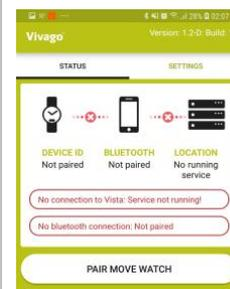
Choose the device ID from the list that represents the watch to be paired. The watch's ID can be found also from the bottom of the watch. After successful pairing, the paired device can be
