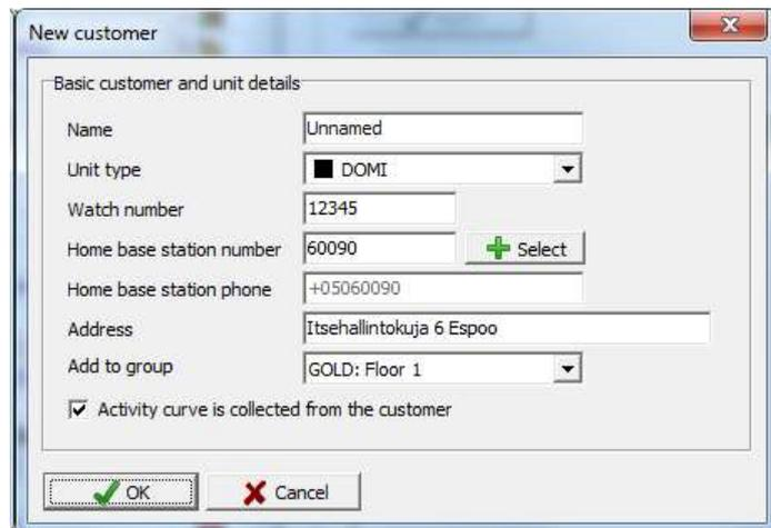
Hint: you can use a barcode or QR code reader to read the watch and base station IDs directly from the devices or the DOMI box. Always confirm the read ID showing in the unit number field matches to the ID printed on the device.
