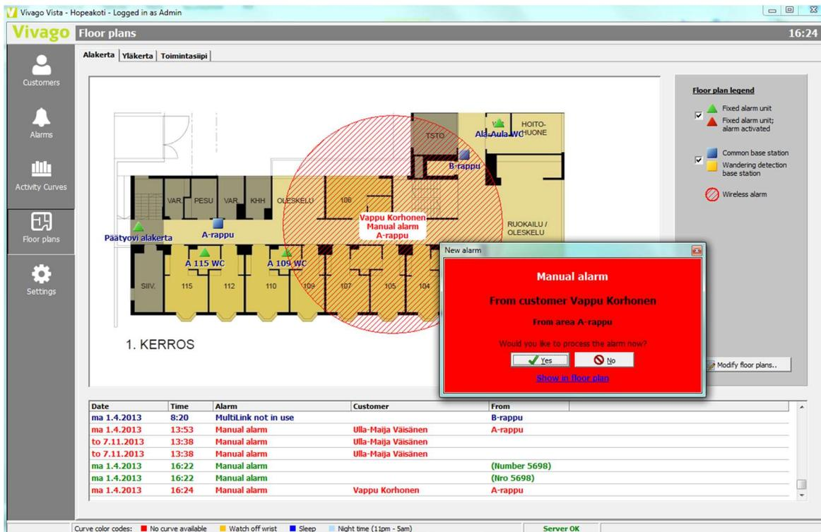
The floor plans view shows a graphical overview of the institutions floor plans. The institution may be split into suitable parts. You can switch between parts (floor plans) by clicking the tabs at the top of the screen. The parts could be different floors of the institutions, different sections and so on.
