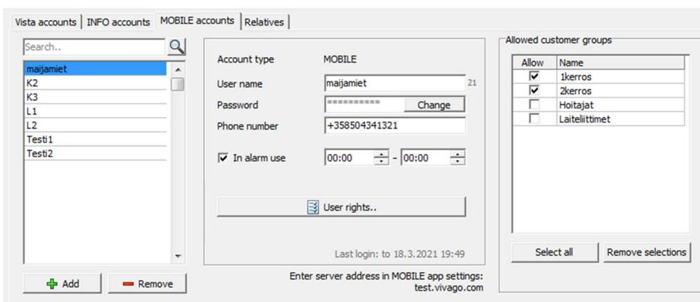
If the MOBILE account is used in a phone or tablet that has a voice connection available, also enter the phone number of the device. Alternatively, you can define the phone number in the MOBILE app's settings. After adding the phone number, you can request a voice connection to the device when acknowledging an alarm from it. Vista will command the customer's voice device (base station) to call the acknowledging device. The voice connection can be opened by simply answering the incoming call.
