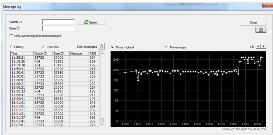
For example, to see all messages and their signal levels (RSSI) from a single watch, fill the Watch ID field but leave the Base ID field empty. Select History above the message list. Click Search. Use the corresponding graph to check how the signal levels of the single watch has changed. Use the left and right arrow buttons on the right side of the screen to change the time scale of the signal level history graph.
