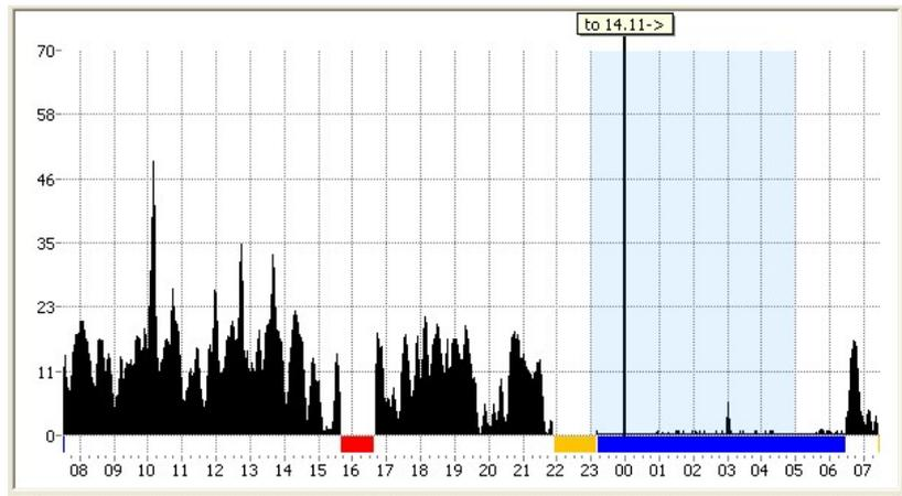
Vista displays activity curves on specific curve screens. There are short-term 60-minute screens and long-term 6 to 24 hour screens in Vista. The bottom edge of the screen displays a timeline, which shows the corresponding time for each point of the screen. On the left side there is a vertical axis with numbers ranging from 0-100%. 100% is the highest possible activity.
